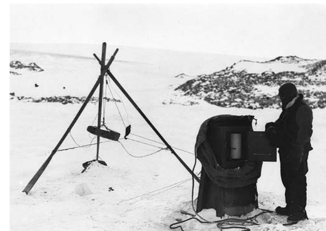
Figure 6. Le marégraphe de Commonwealth Bay en 1912. ©AAD The Commonwealth bay tide gauge in 1912.
